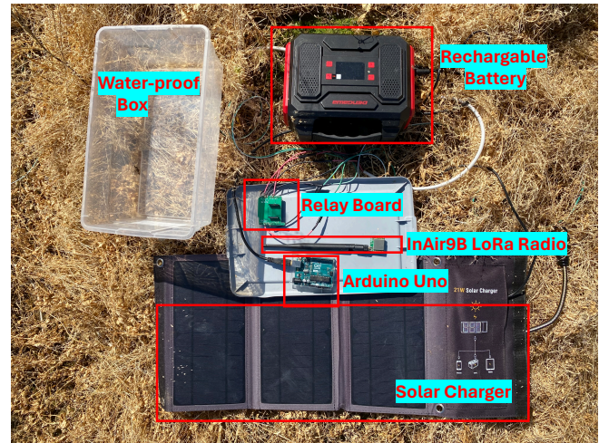
Figure 13: The illustration of the solar-powered sensor node.
